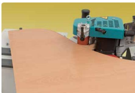
Automatic rear tape cutting. Foot pedal for curved or shaped pieces.
